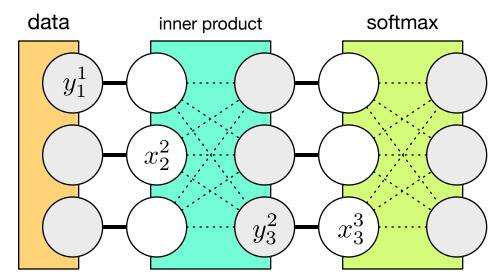
Each layer is now represented as a *box* that has inputs (denoted by  $x^L$  for the L-th layer) and outputs (denoted by  $y^L$ ). Now the architecture specifies which layer's outputs connect to which layer's inputs (the dark lines in the figure). On the other hand, the intra-layer connections, or computations (see dotted line in the figure), should be isolated from the outside world.
