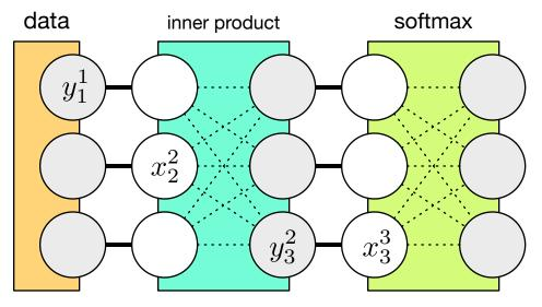
Each layer is now represented as a *box* that has inputs (denoted by  $x^L$  for the *L*-th layer) and outputs (denoted by  $y^L$ ). Now the architecture specifies which layer's outputs connect to which layer's inputs (the dark lines in the figure). On the other hand, the intra-layer connections, or computations (see dotted line in the figure), should be isolated from the outside world.
